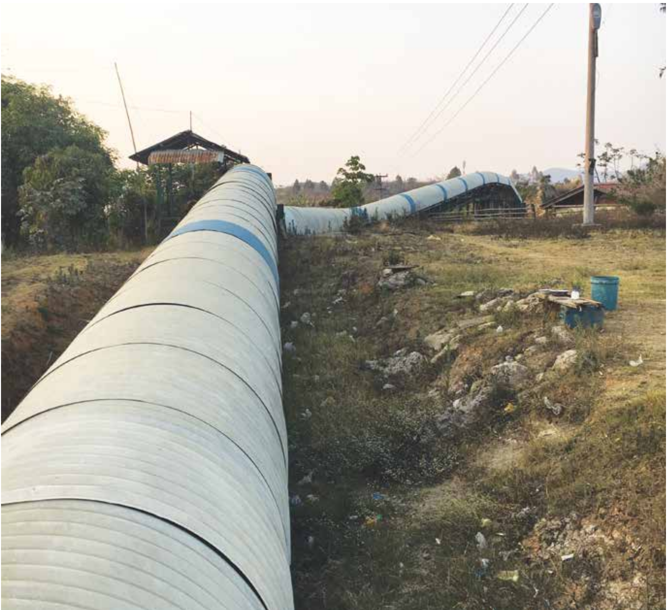
The conveyor belt was used to transfer coal from Tigyit mine to the thermal power plant
