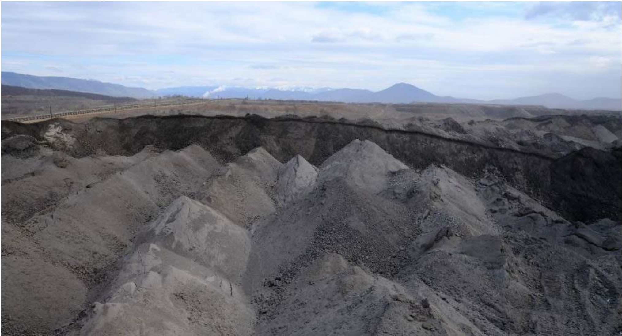
Freshly deposited external overburden dump, TPP in the background Kardia Mine, West Macedonia, Greece
